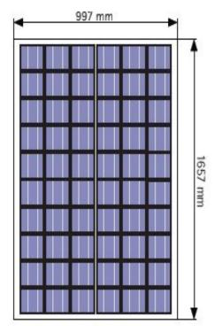
Rated value with nominal operating cell temperature (NOCT:800 W/m²,48± 2°C,spectrum AM 1.5)
